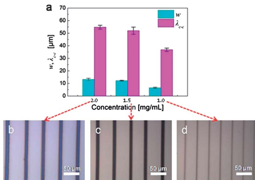
**Fig. 3** (a) The variation in PMMA pattern width ( $w$ ) and the distance between neighboring stripes ( $\lambda_{c-c}$ ) as a function of PMMA concentration. The microscope images show the resulting patterns formed at PMMA concentrations of (b) 2.0, (c) 1.5, and (d) 1.0  $\text{mg mL}^{-1}$ .
