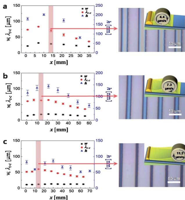
**Fig. 2** The variation of PMMA pattern width ( $w$ ), the distance between neighboring stripes ( $\lambda_{c-c}$ ) and the height ( $h$ ) as a function of the distance ( $x$ ) from the initial pattern. The roll moving speed was (a) 4.4, (b) 7.3, and (c) 11.2  $\mu\text{m s}^{-1}$ . The microscope images of the PMMA patterns at the same location ( $\sim 14$  mm from the initial pattern) are also displayed. The inset illustrates the pattern formation with respect to the roll moving speed.
